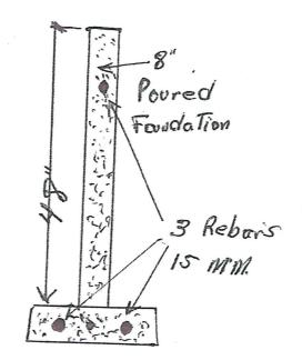
6×18" Footing on undisturbed soil
