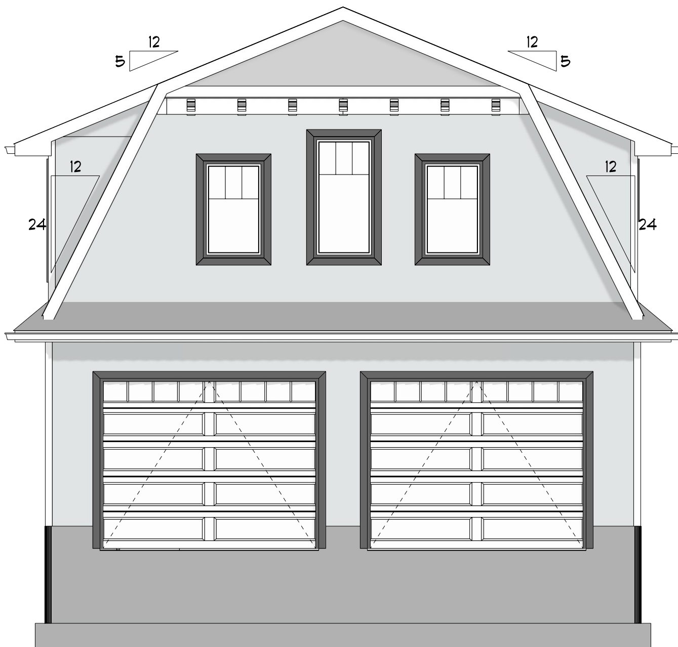
GARAGE ROAD SIDE SCALE: 1/4" = 1'-0"
