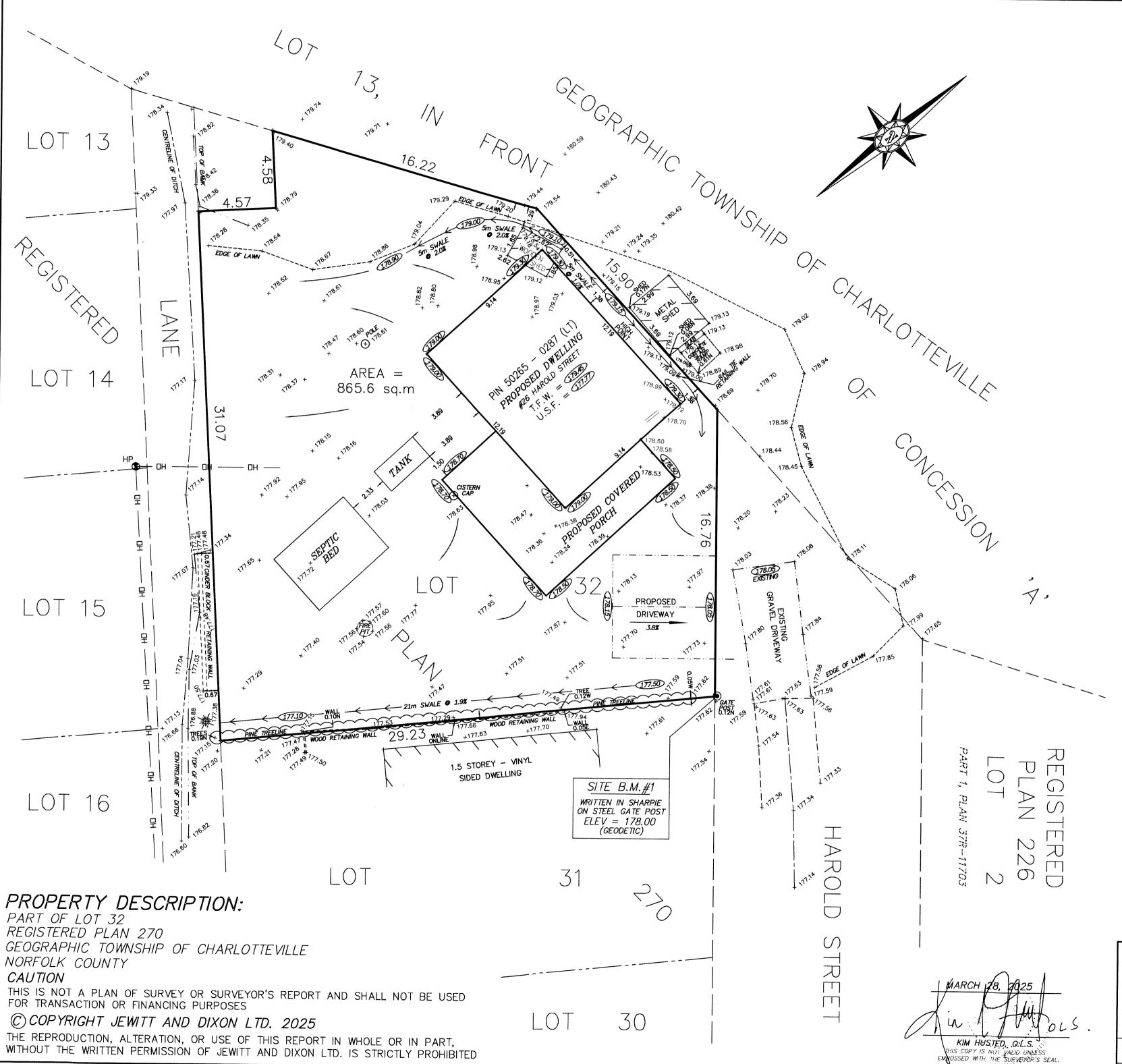
PROPOSED LOT GRADING AND DRAINAGE SITE PLAN
