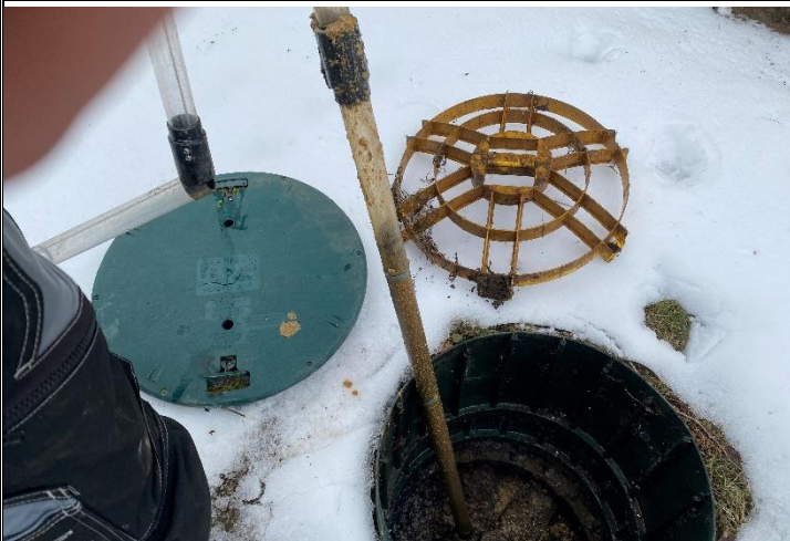
5. Septic tank solids accumulation measurement – pump out required
