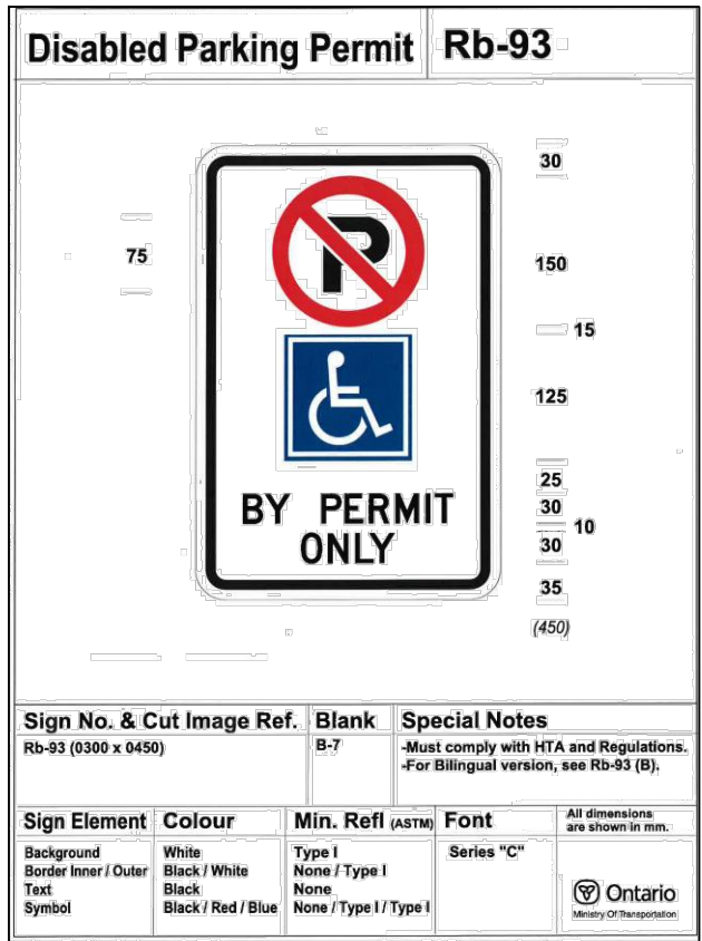
BARRIER FREE PARKING SIGN DETAIL N.T.S.
